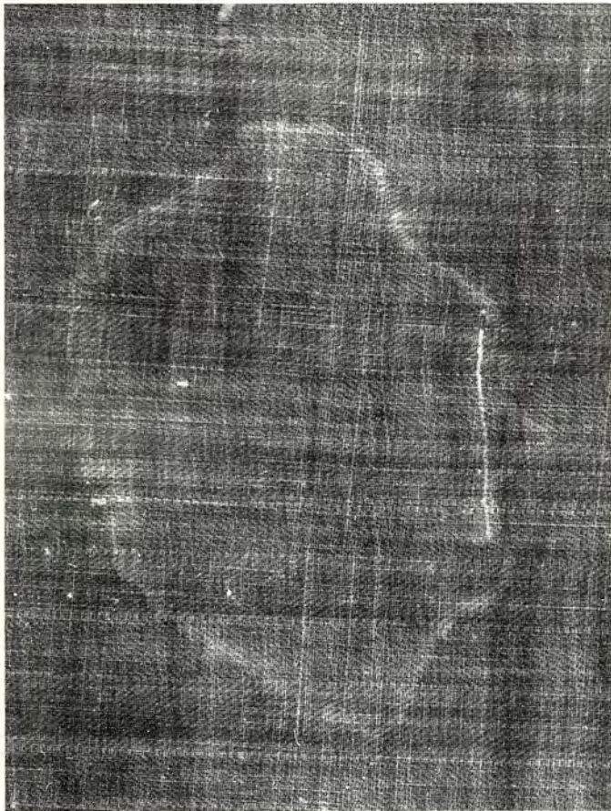
Figure 2—Radiographic image of one of many water stains. Also visible is the herringbone pattern of the linen.
